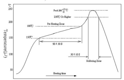
Remark1:Recommended IR Reflow Soldering Profile meet J-STD-020D. Remark2:The peak temperature of soldering heat is 260 +5/-0℃ for 10 seconds
